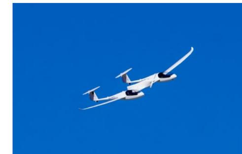
HY4 - first four-seater passenger aircraft powered solely by a hydrogen fuel cell battery system (DLR)
