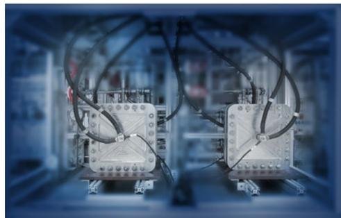
Polymer electrolyte membrane-based stack combination used for characterization in electrolysis test stand (FZJ)
